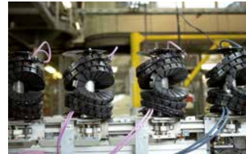
Test for torsion and twisting with e-chains® and chainflex® cables
